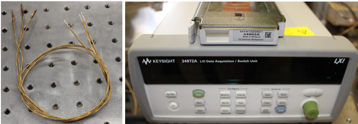
Figure 4.2: Thermocouples (left), and the data acquisition system (right) used in the experiment.
